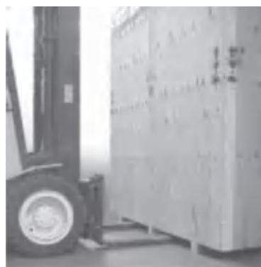
Figure 21 Lifting switchgear packed in a wooden crate
