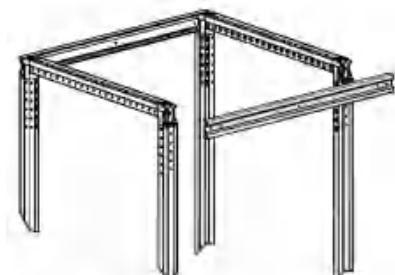
upper removable cross-member to simplify connection
